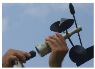
Connect the cable to the sensor.
