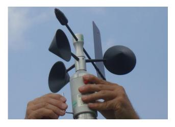
Mount the sensor on the mast and tighten the screw.
