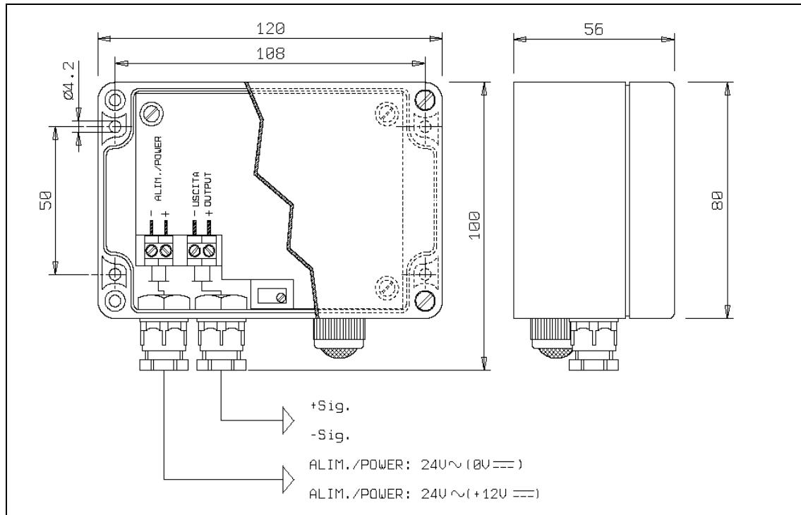
APPENDICE B – Ingombro e connessioni per modelli DQA22x / Overall dimensions and connections for DQA22x models
