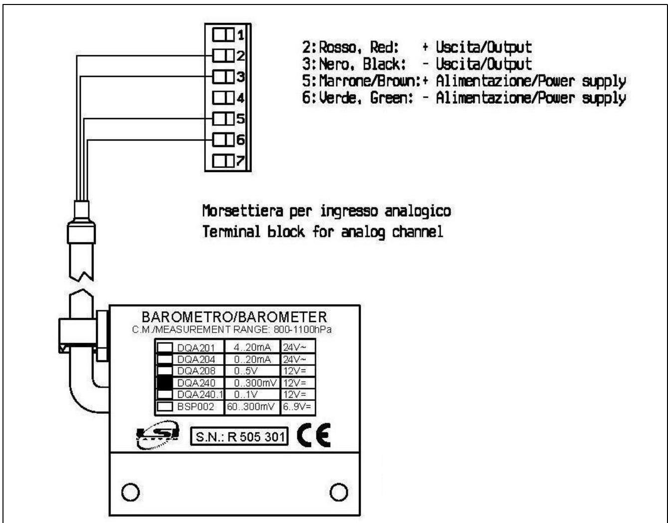
**APPENDICE F – Connessione sensore DQA240.1 ad acquisitore LSI LASTEM E-Log / Connection between DQA240.1 sensor and LSI LASTEM datalogger E-Log**
