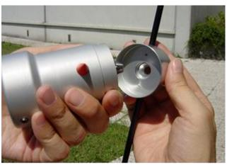
Insert the wind vane on the sensor's body. Take care to centre the wind vane's notch with the tooth on the sensor body's rotating cone.
