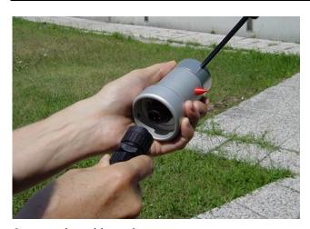
Connect the cable to the sensor.
