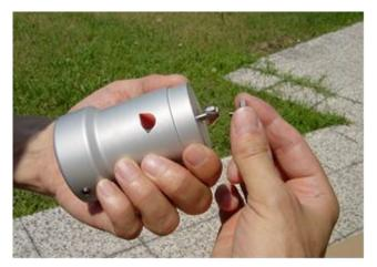
Unscrew the screw from the shaft thread.
