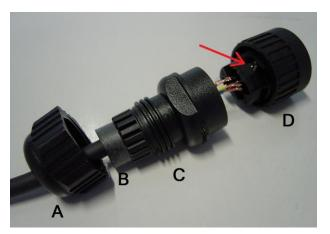
DNA212 comes with MG2257 free connector. Pass the cable as in the picture above, select the rubber ring B (ø 6 or 9 according to the cable dimension). Then fix the wires to the connector as in the drawing on the left. Read also DISACC 5635 drawing.
