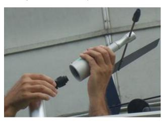
Connect the cable to the sensor.
