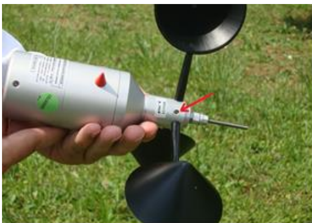
Tighten the screw of the rotor (indicated by the arrow).
