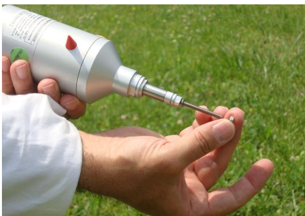
Unscrew the nut and washer from the shaft thread.
