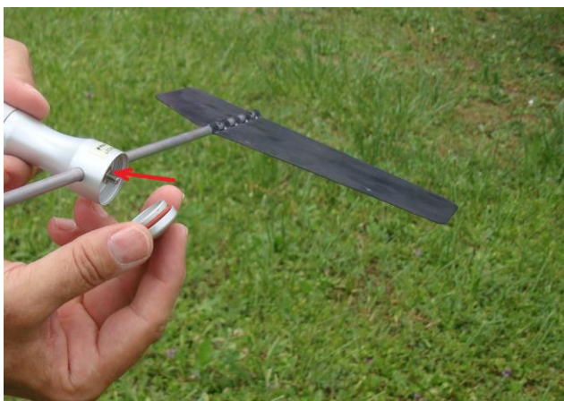
Fix the top (indicated by the arrows) and tighten it .
