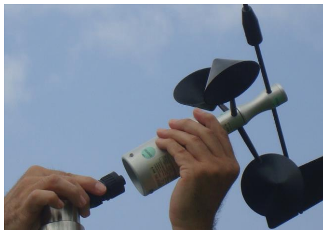
Connect the cable to the sensor.
