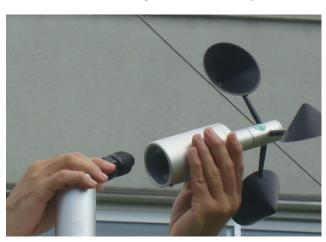
Connect the cable to the sensor.
