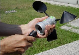
Connect the cable to the sensor.
