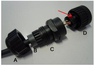
DNA202 comes with MG2257 free connector. Pass the cable as in the picture above, select the rubber ring B (ø 6 or 9 according to the cable dimension). Then fix the wires to the connector D.
